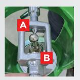
First slide the back part of the regulator onto the cylinder valve. On its upper part this has a tightening screw (marked as A) and on its lower part this has a rubber washer (known as a 'Bodok Seal', and marked as B).
