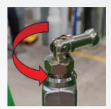
Now open the valve of the cylinder **slowly** by hand using the toggle as a lever and turning it at least ½ full turn. Now you will notice that the gauge on the regulator is no longer at 'O' but rather is marking the level of oxygen in the cylinder. NO SOUND OF LEAKS SHOULD BE HEARD!
